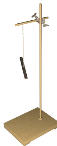
Fig. 10.9 A freely suspended bar magnet always comes to rest in the same direction
