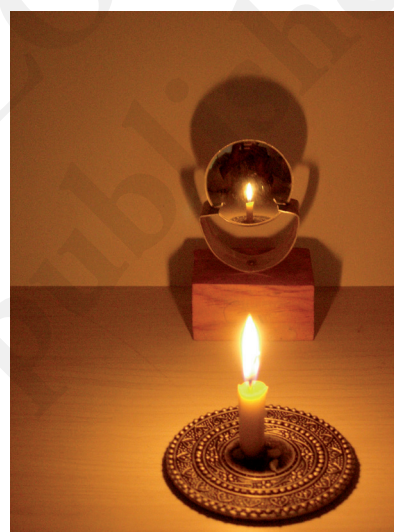
Fig. 11.19 Image formed by a convex mirror
