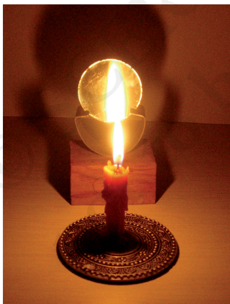
Fig. 11.16 Virtual image formed by a concave mirror
