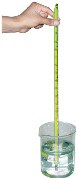
Fig. 3.5 Measuring temperature of water with a laboratory thermometer
