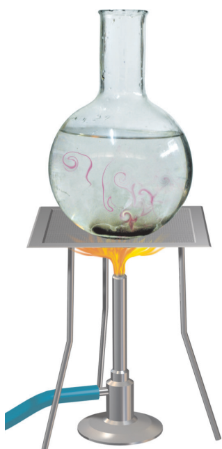
Fig. 3.9 Convection of heat in water
