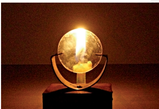
Fig. 11.26 Virtual image formed by the convex lens
