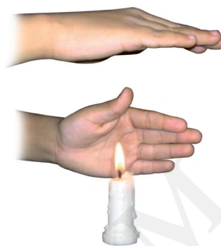
Fig. 3.10 Transfer of heat by convection in air
