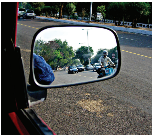
Fig. 11.20 Convex mirror as side view mirror
