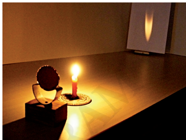
Fig. 11.15 Real images formed by a concave mirror
