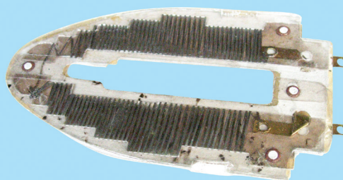
Fig. 10.11 Element of electric iron
