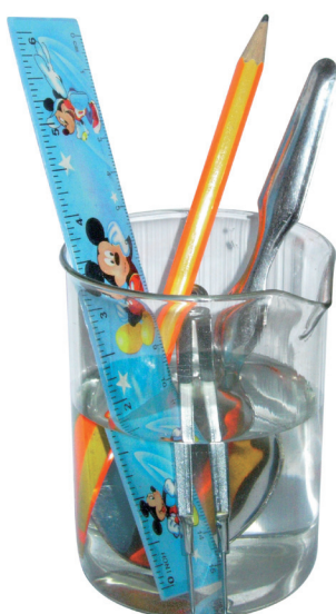
Fig. 3.8 Conduction of heat by different materials
