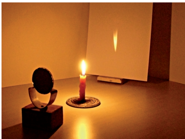
Fig. 11.15 Real images formed by a concave mirror
