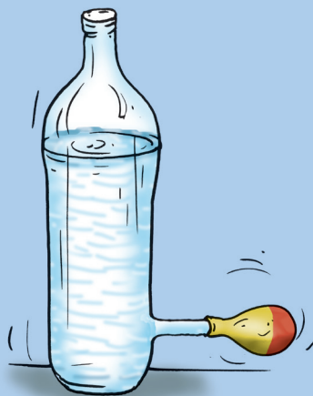
Fig.8.15 : A liquid exerts pressure on the walls of the container
