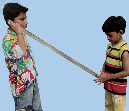
Fig. 10.12 : Sound travelling through a metre scale
