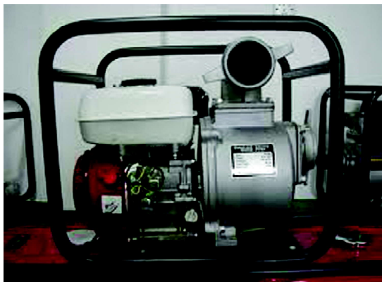
A water pump
